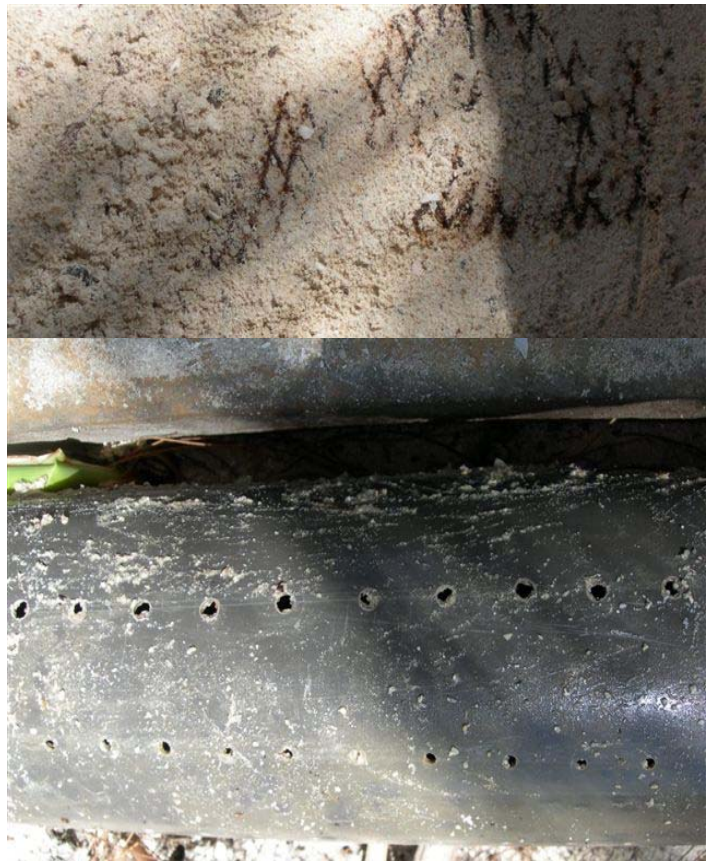
Figure 2. The rusty mesh (above) and the pipe with non-clogged holes (below)
